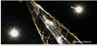
Roccor's helical L-band antenna is helping the Air Force Research Laboratory's XVI mission to demonstrate communications relay with a Link 16 terminal on a small satellite.
